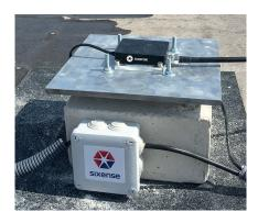
4DBloc has been developed and tested in co-operation with the French National Institute of Geographic and Forest Information (IGN) with the aim of creating a **GNSS-based position measurement system** that is simple, to deploys, robust, autonomous and accurate.
