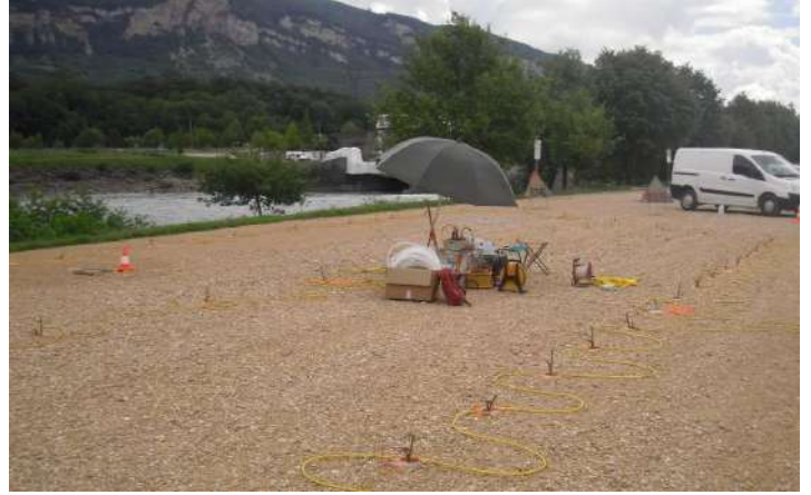
Measuring device for the electrical tracing method
